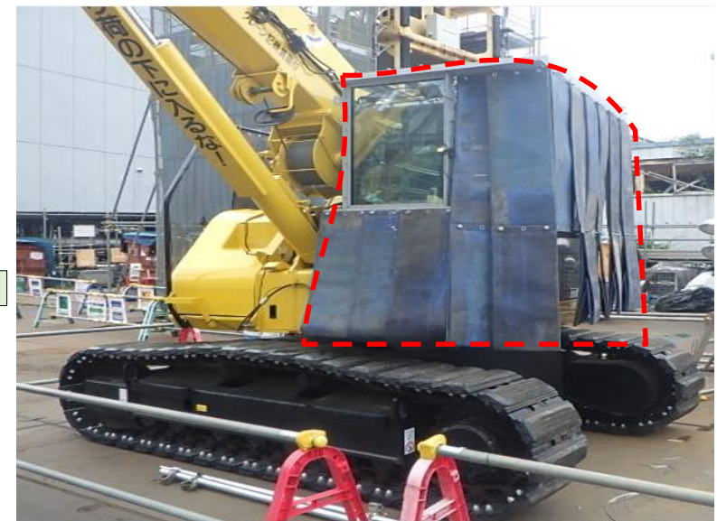
Crane after installation of lead shielding and flint glass (photographed on May 22, 2025)
