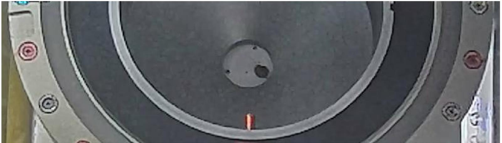
The sampled fuel debris at the bottom of the transportation box (April 22)
