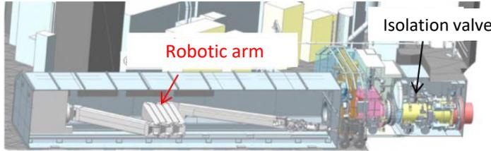
8. Internal investigation/debris sampling using robotic arm
