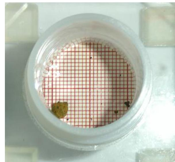
Fuel debris sample in a specimen container inside the glove box
