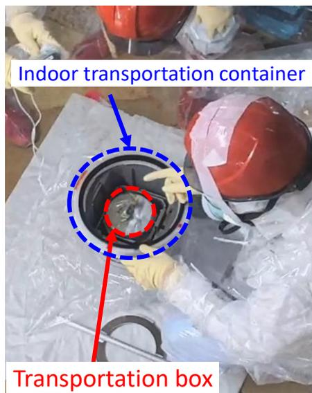
Loading the transportation box into an indoor transportation container
