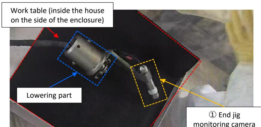
Replaced ① End jig monitoring camera
