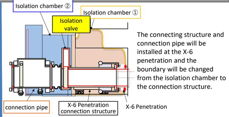
5. Installation of telescopic device
