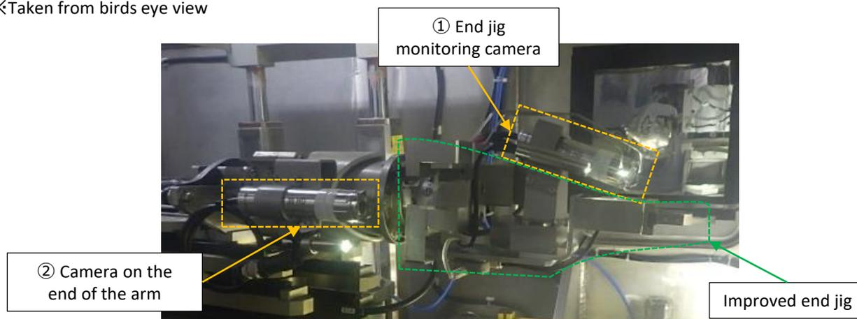
Replaced cameras ① ② and improved end jig
