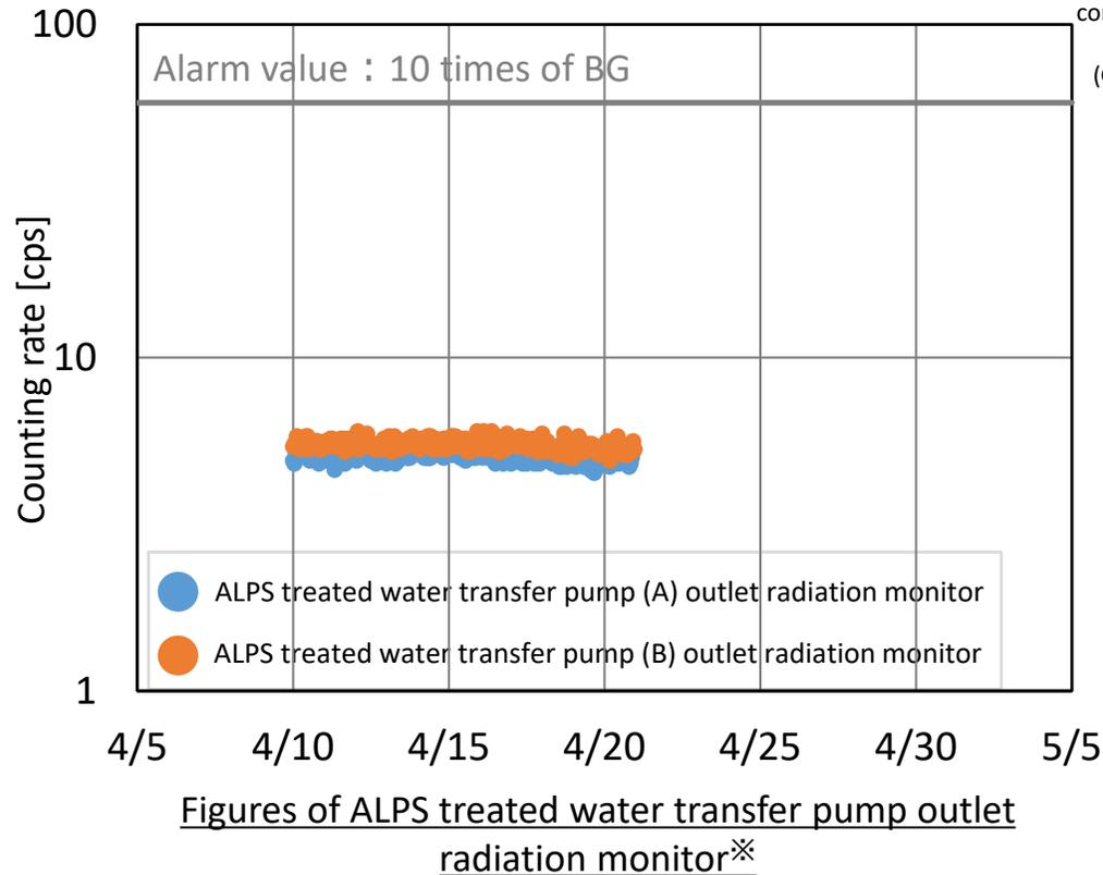
※ : As shown in the schematic on the upper right, ALPS treated water was passed through System B. (System A was filled with filtrated water)
