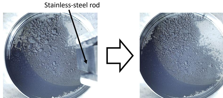
Specimen preparation (uniform powder mixture)
