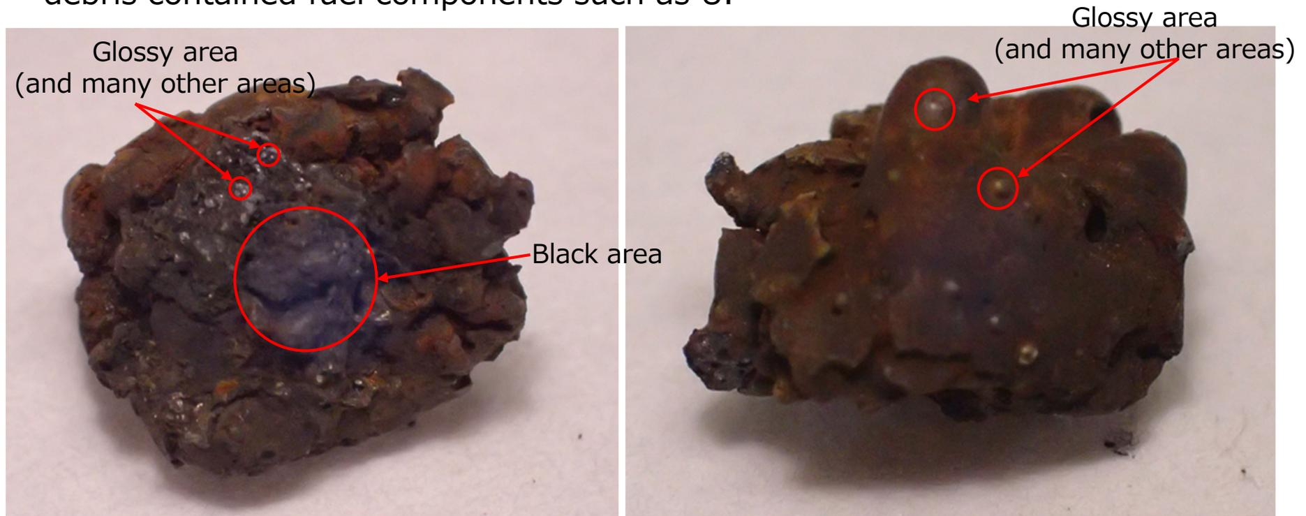
Enlarged photo of External appearance of fuel debris sample [1]
