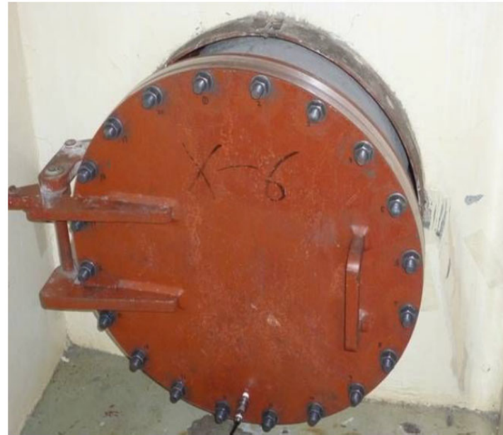
Photo from flange leak tests
