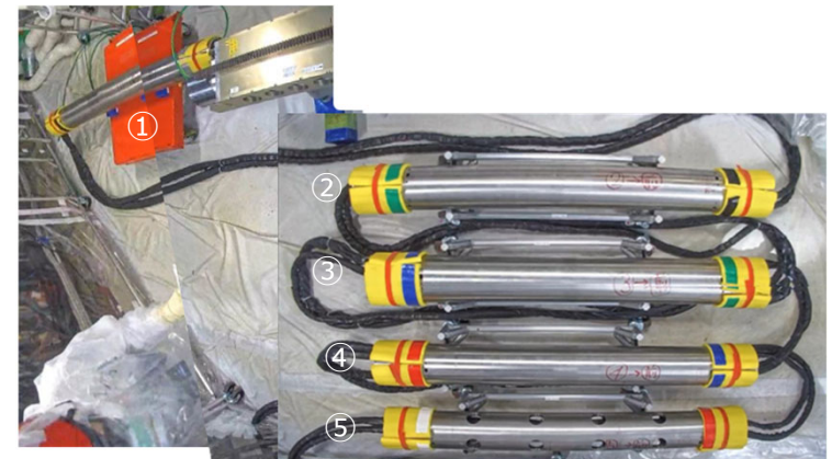
Rearranging push pipes in their correct order at the Fukushima Daiichi Nuclear Power Station site (Photographed between September 7-September 8, 2024)
