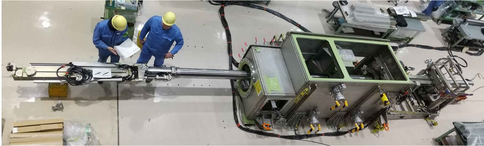
Telescopic trial retrieval equipment (photo taken from above the equipment)
