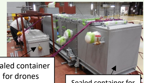
Sealed container for snake-like robot
