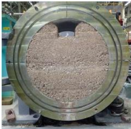
Conditions inside the X-6 penetration (mockup)
