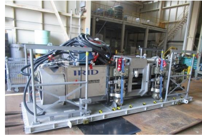
Exterior view of the deposit removal equipment (high pressure water/abrasive water jet)
