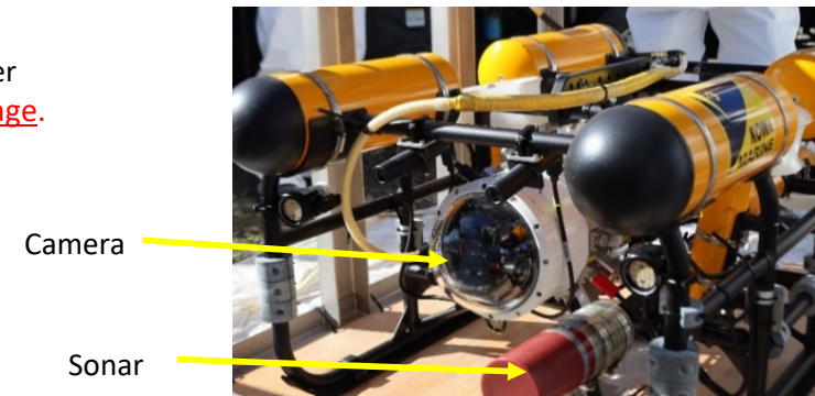
ROV used for the inspection Dimensions: 1,036mm×720mm×630mm Mass: Approx. 75kg
