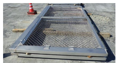
Main installation net to prevent the fish from leaving (Mesh size of 5 cm)
