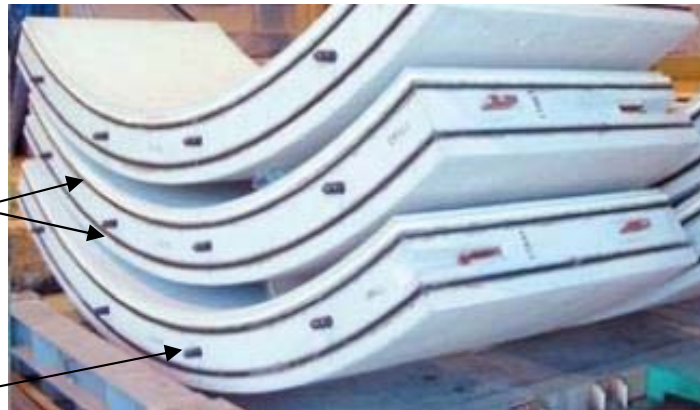
Reinforce concrete tunnel walls (segments)
