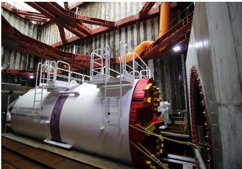
Shield machine storage
