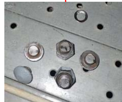
Bolts at the joint ruptured
