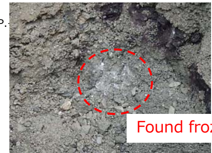
Excavated soil (Solidified) (Measurement point① Near G.L.-1.3m)
