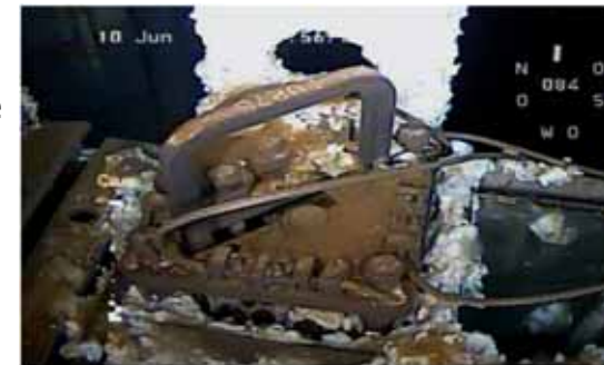
TOP of wire-repaired fuel
