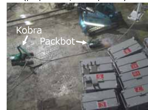
Engaging in preparations using small robots (Kobra, Packbot)
