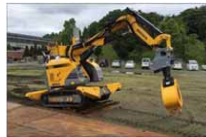
Remotely operated heavy machinery (BROKK)
