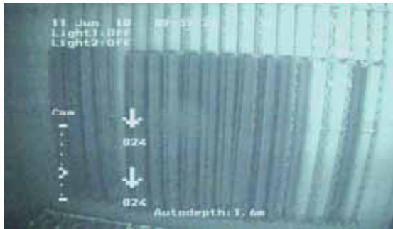
Control rods and control rod hangers
