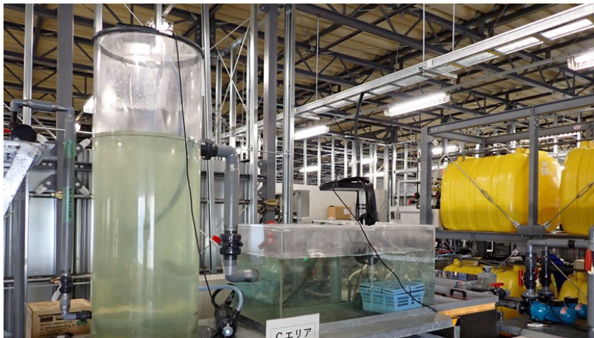
Seaweed tank removed from isolation. Yellowish seawater inflow from flounder and abalone tanks.
