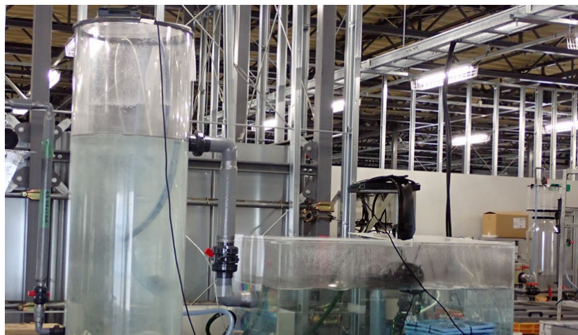
Isolated seaweed tank. Sterilized with ultraviolet (UV) light and purified with active carbon.
