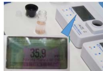
The samples show chromogenic reaction depending on its nitric acid concentration. (The measurement value is 35.9mg-NO 3 /L at this time)
