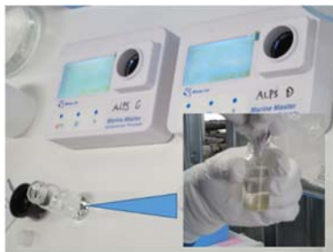
Sample rearing water into a cuvette and add reagent to it.
