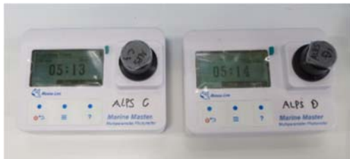
Leave the cuvette to stand for designated time period. (measuring equipments show time)
