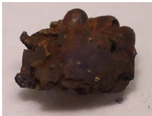
External appearance of fuel debris sample (Approx. 9mm x 7mm)
