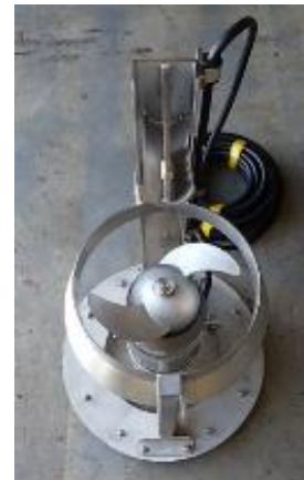
Agitator to be installed in the tanks used for measurement and confirmation purposes TEPCO
