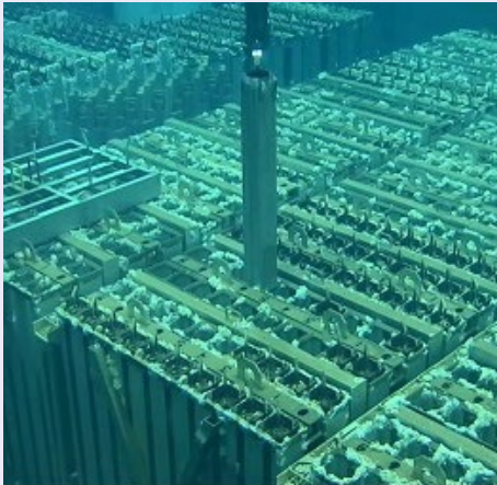
< Unit 2 fuel removal training showing mockup fuel being hoisted (photo taken on May 13) >
