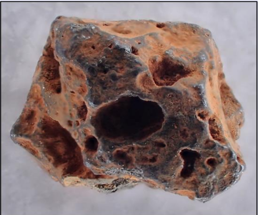
Enlarged photos showing the external appearance of the fuel debris sample (taken from directly above)
