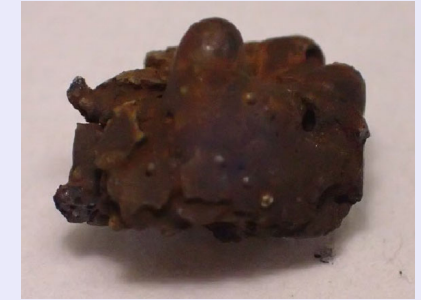
< External appearance of fuel debris sample (approx. 9 × 7 mm) >
