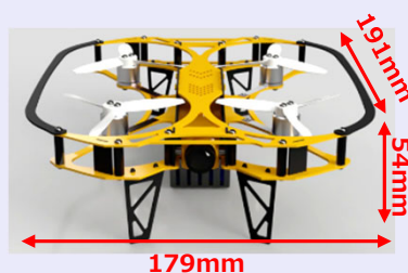
< Small drone used in the investigation in Unit 1 >
