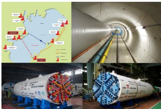
Shield method (Tokyo Electric Power Co., Inc., 2009) East-West Joint Gas Pipeline Tunnel at the Transverse Section of Tokyo Bay: Approx.18 km
