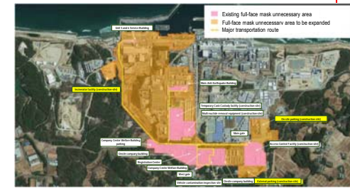
In May 2013, areas excluding those around Unit 1-4, tank areas and rubble storage areas were set to full-face mask unnecessary areas.
