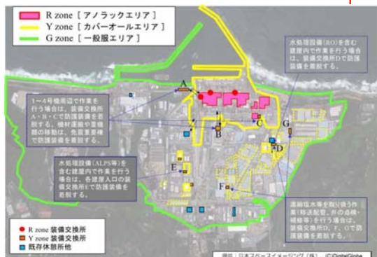
In March 2016, based on the progress of measures to reduce the environmental dosage on site, the site was categorized into two zones: Highly contaminated area around Unit 1-4 buildings, etc. and other areas where limited operation started to optimize protective equipment according to each category.
