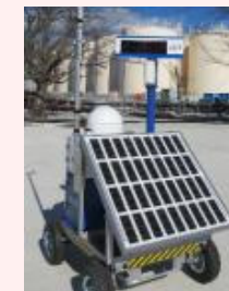
Installation of Dose-rate monitor
