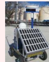
Installation of Dose-rate monitor
