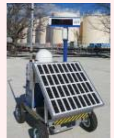
Installation of Dose-rate monitor
