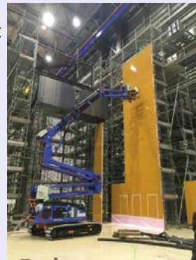
<Decontamination of mockup high-place wall>
