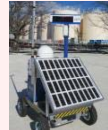
Installation of Dose-rate monitor
