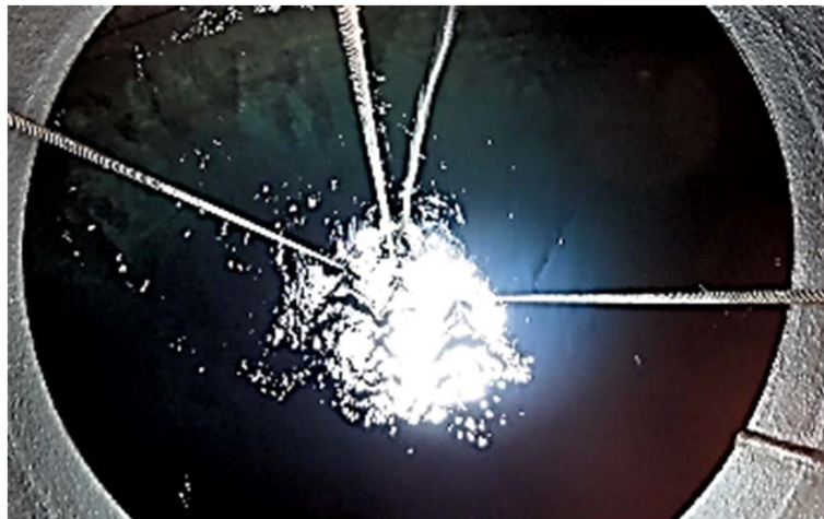
Tank water surface when agitator is running (photographed at T/R)
