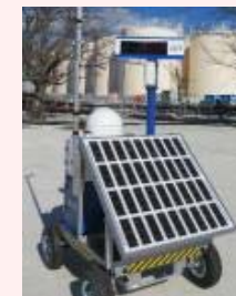
Installation of Dose-rate monitor
