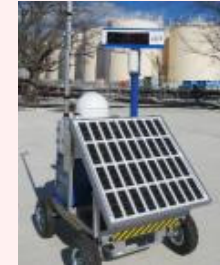
Installation of Dose-rate monitor
