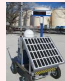
Installation of Dose-rate monitor
