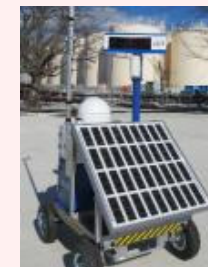
Installation of Dose-rate monitor
