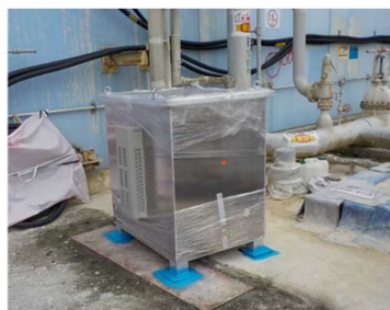
Muon measurement equipment (Small device, about 1m x 1m x height 1.3m)
