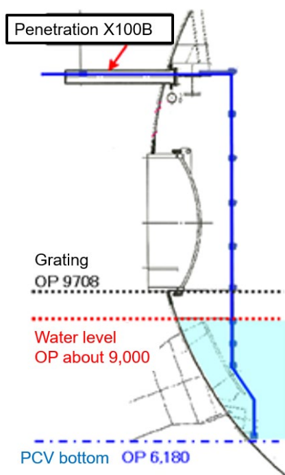
Figure 4.2.1-2 Residual water level measurement results in Unit 1 D/W [1-4]
