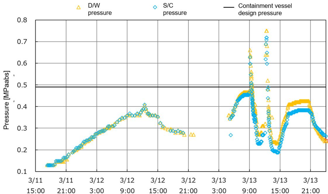
Figure 13 Containment vessel pressure (from 15:00 on the 11th to 00:00 on the 14th)
