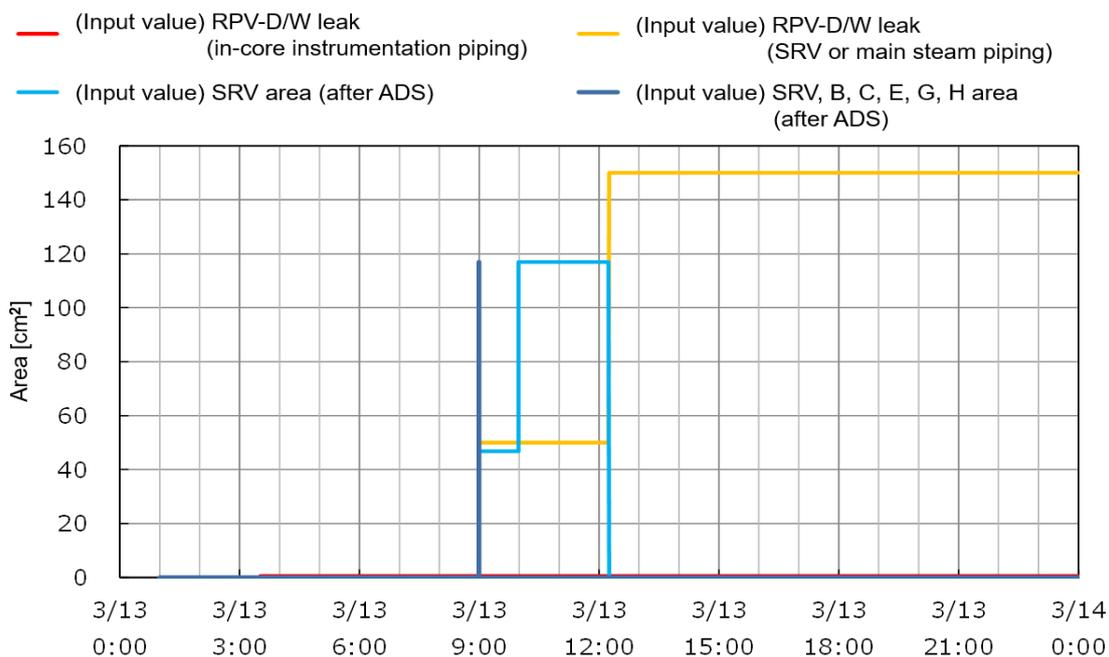
Figure 16 Gas phase leakage area from pressure vessel and SRV opening area (per valve) (evaluation case with a large amount of hydrogen formation)
