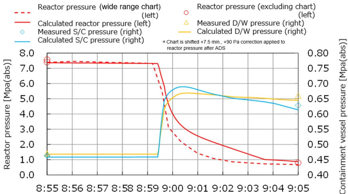
Figure 21 Analysis results of reactor pressure and containment vessel pressure (30 cm<sup>2</sup> pressure vessel gas phase leak)
