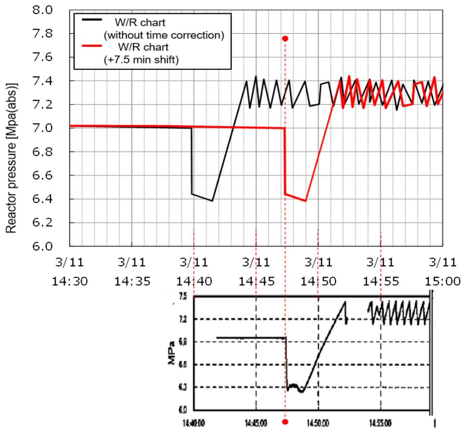
Figure 4 Relationship between reactor pressure wide range chart data before and after scram and reactor pressure data from transient recorder (only time correction applied)
