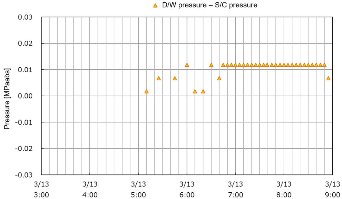
Figure 9 Pressure difference between D/W and S/C before ADS activation
