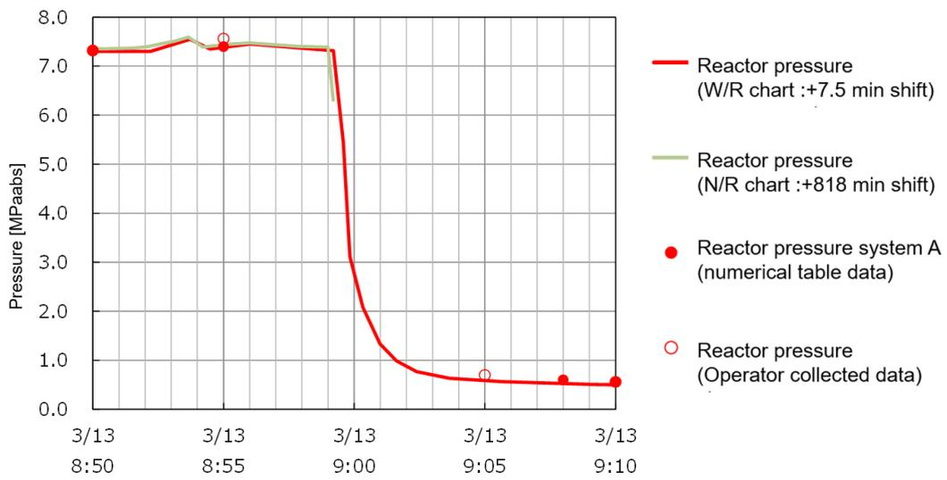
Figure 8 Reactor pressure before and after 09:00 on the 13th (only time correction applied)
