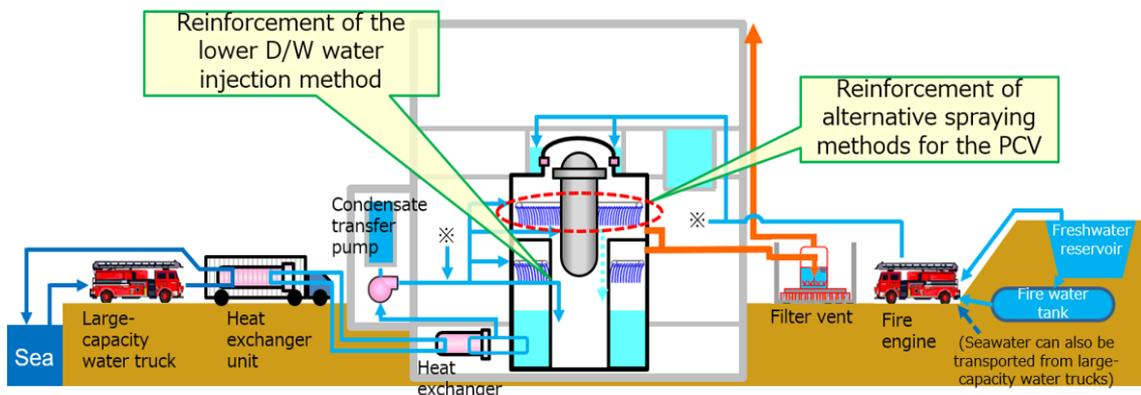
Figure 24 Measures to prevent PCV damage at the Kashiwazaki-Kariwa NPS (conceptual diagram)
