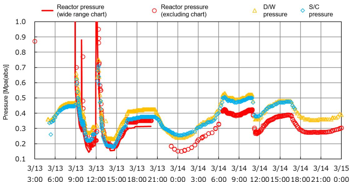
Figure 2 Measured reactor pressure and containment pressure of Unit 3 (uncorrected) (Data in the chart are digitized and illustrated; the same applies to the following figures.)
