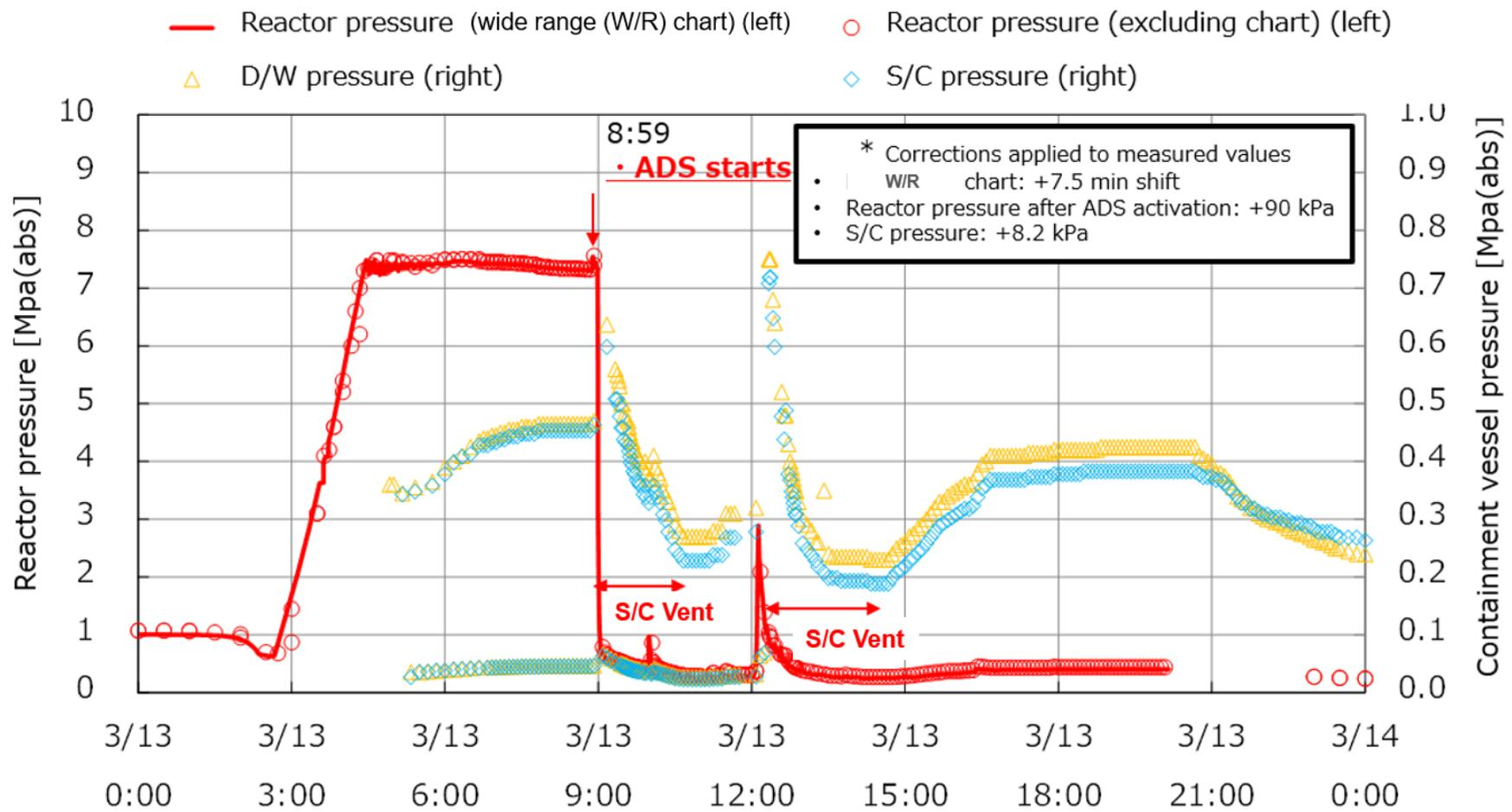
Figure 1 Developed accident progression scenario
