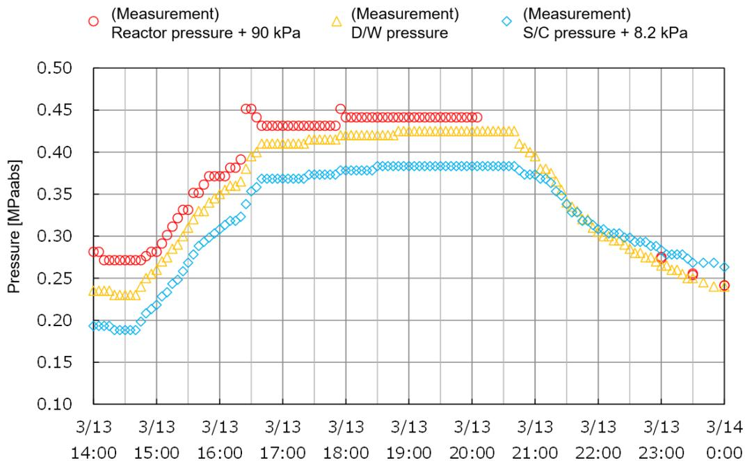
Figure 14 Containment vessel pressure and reactor pressure (from 14:00 on the 13th to 00:00 on the 14th)
