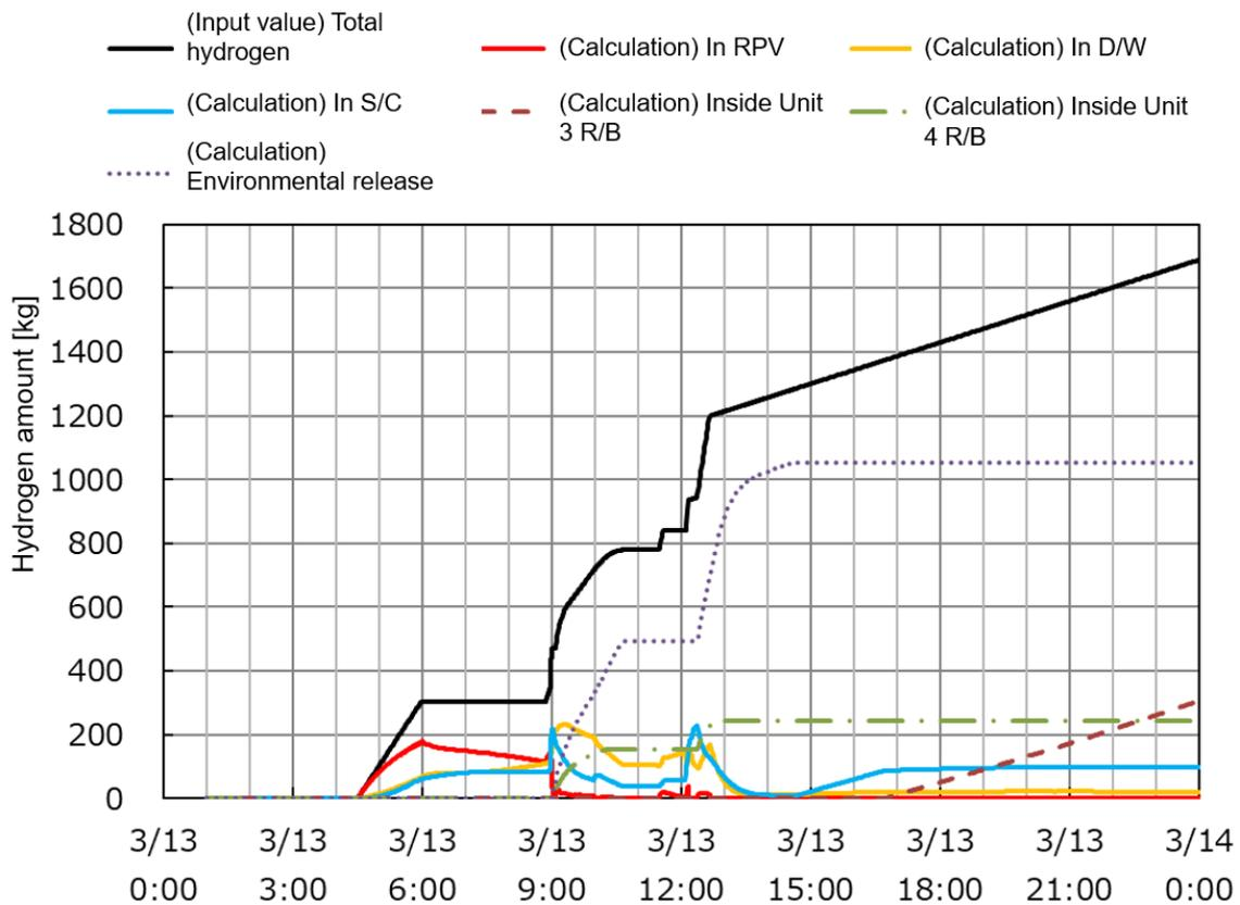
Figure 20 Results of analysis of hydrogen abundance at various locations (evaluation case with a large amount of hydrogen formation)
