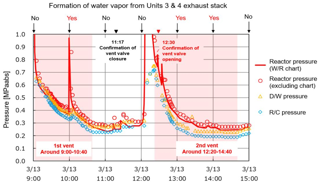
Figure 12 Containment vessel pressure behavior; presence or absence of water vapor release from the exhaust stack (Correction: chart +7.5 minute shift, reactor pressure +90 kPa, S/C pressure +8.2 kPa)
