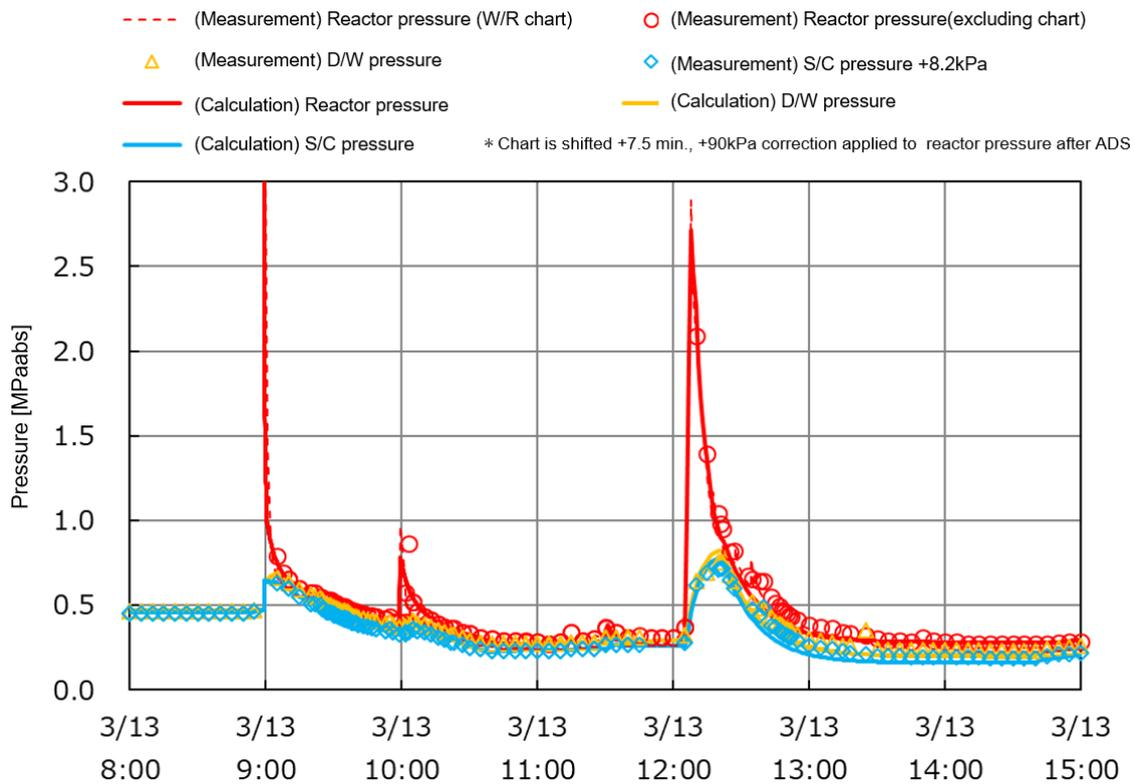
Figure 23: Analysis results of reactor pressure and containment vessel pressure (SRV fully closed case)
