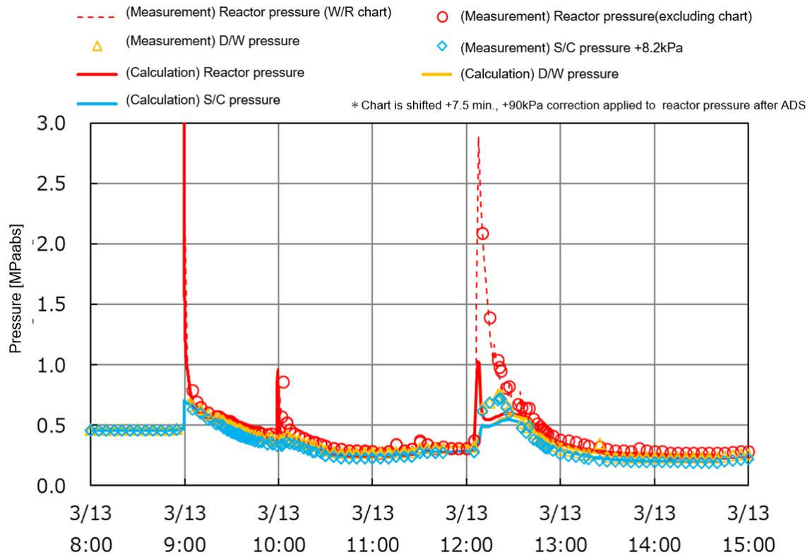
Figure 22 Analysis results of reactor pressure and containment vessel pressure (SRV6 valves maintained open case)
