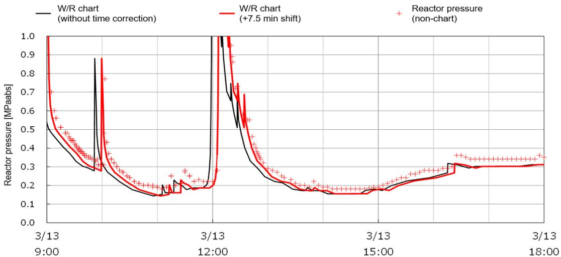
Figure 5 Relationship between reactor pressure wide range chart data and reactor pressure data other than chart data after 09:00 on the 13th (only time correction applied)
