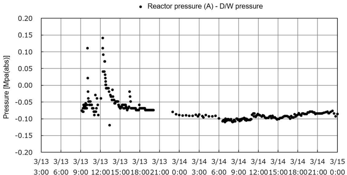
Figure 3 Difference between measured reactor pressure and D/W pressure
