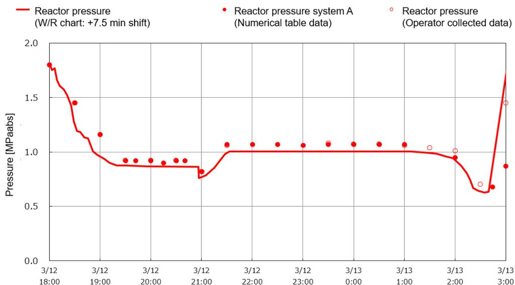
Figure 6 Reactor pressure from 18:00 on the 12th to 03:00 on the 13th
