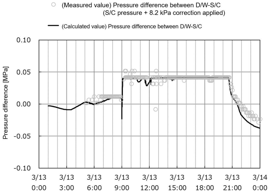
Figure 19: Analysis results of pressure difference between D/W and S/C (evaluation case with a large amount of hydrogen formation)
