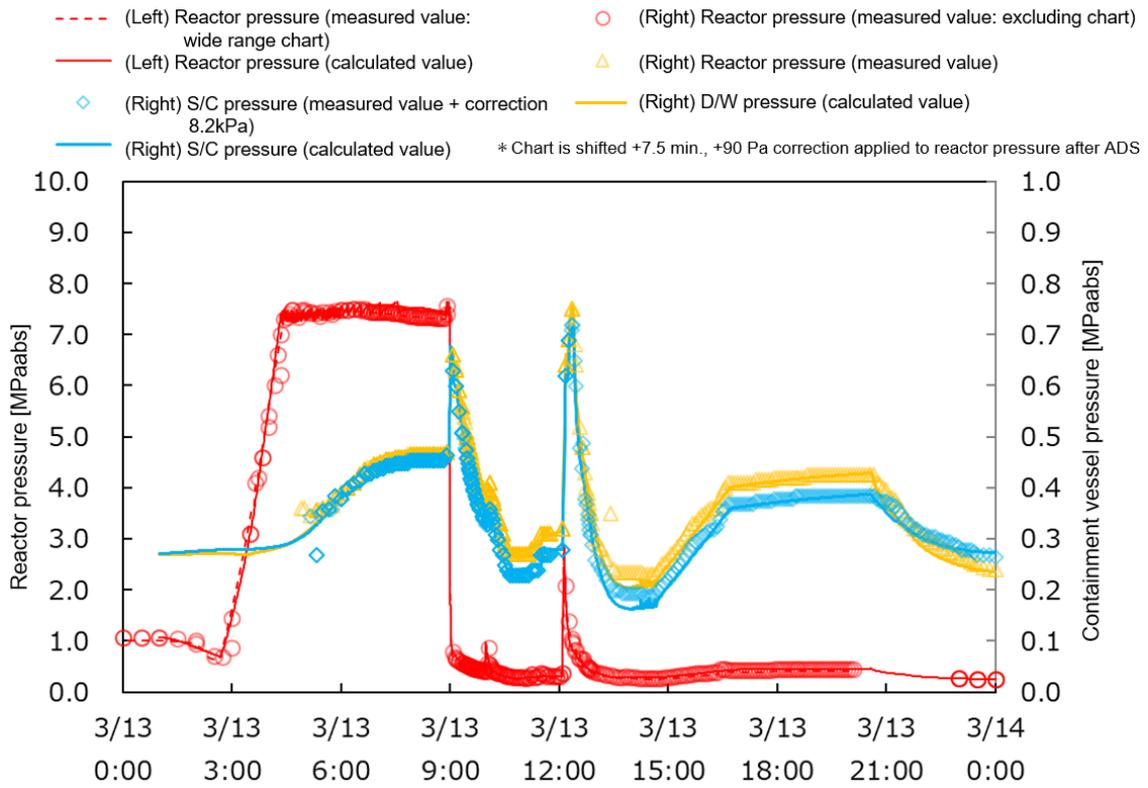
Figure 18: Analysis results of reactor pressure and containment vessel pressure (evaluated case with large amount of hydrogen formation evaluated)
