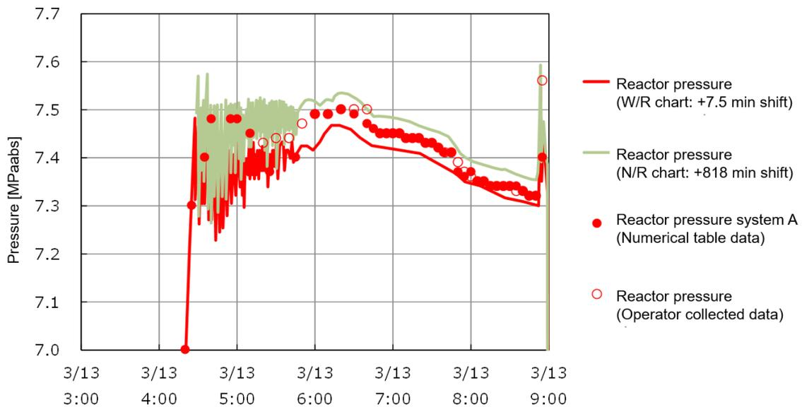
Figure 7 Reactor pressure data from 03:00 to 09:00 on the 13th (only time correction applied)
