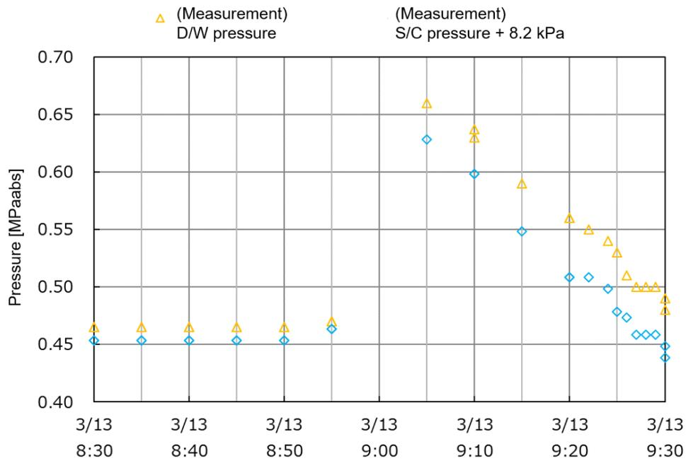
Figure 10 Containment vessel pressure before and after ADS activation
