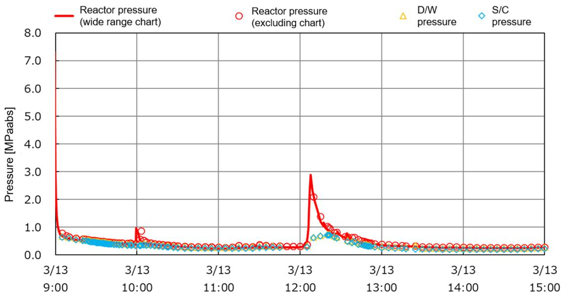
Figure 11 Reactor pressure after ADS activation
