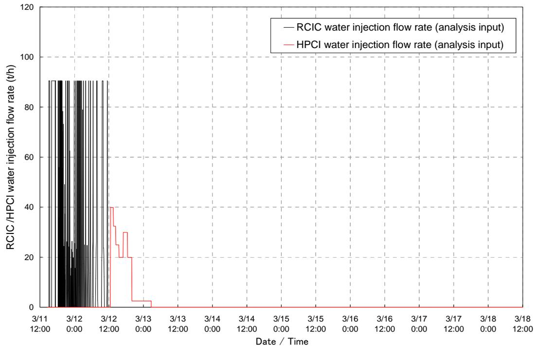
Figure 1 RCIC and HPCI water injection flow rates
