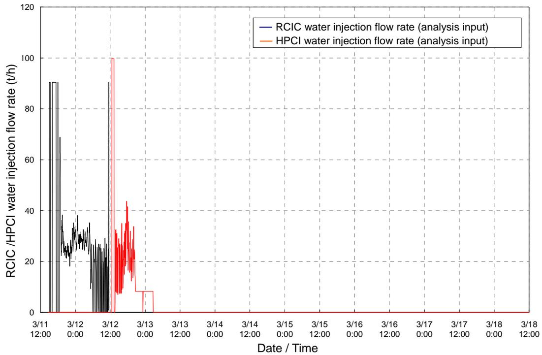
Figure 3 RCIC and HPCI water injection flow rates
