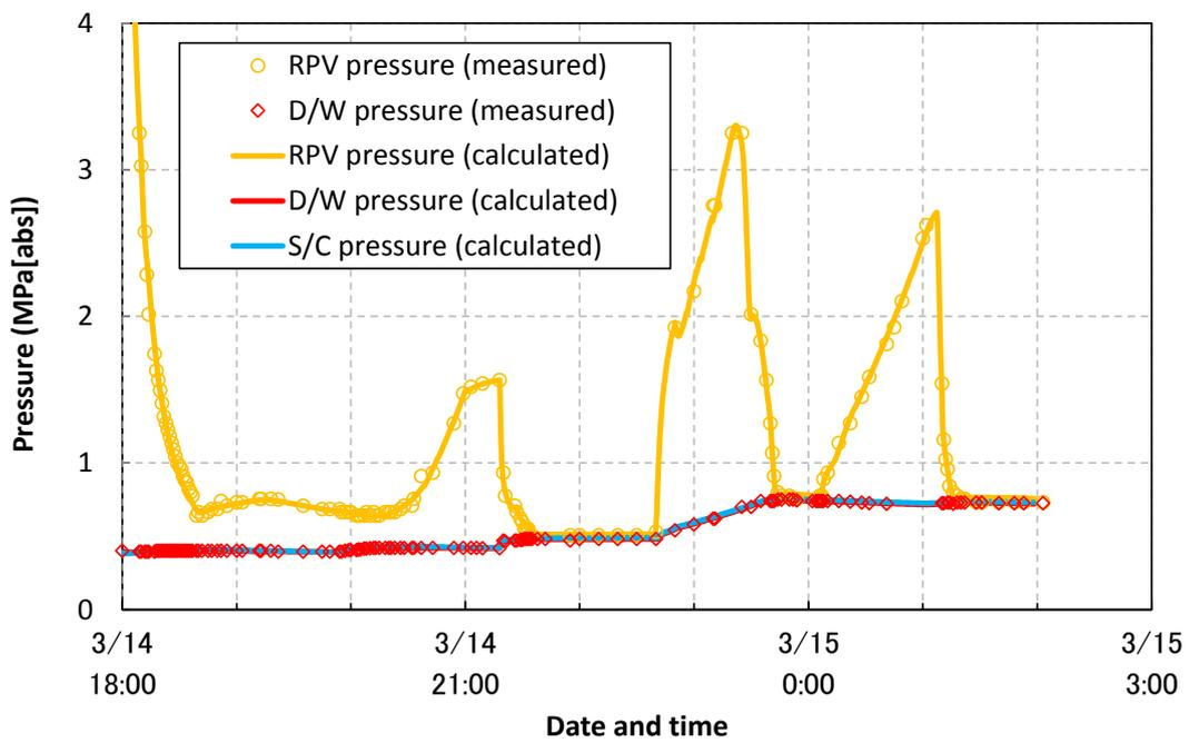
Figure 2-5 Base Case analysis results (Pressure): 0 – 4MPa
