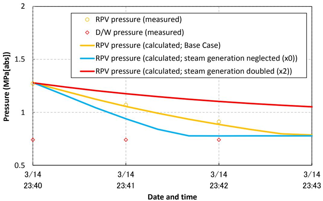
Figure 2.18 Results of Sensitivity Analysis Case ⑤ (RPV pressures)
