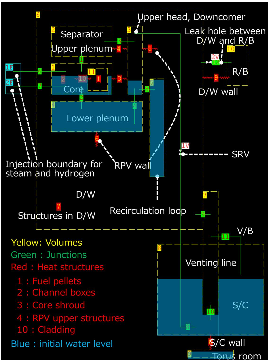
Figure 2.2 Geometry for GOTHIC analysis
