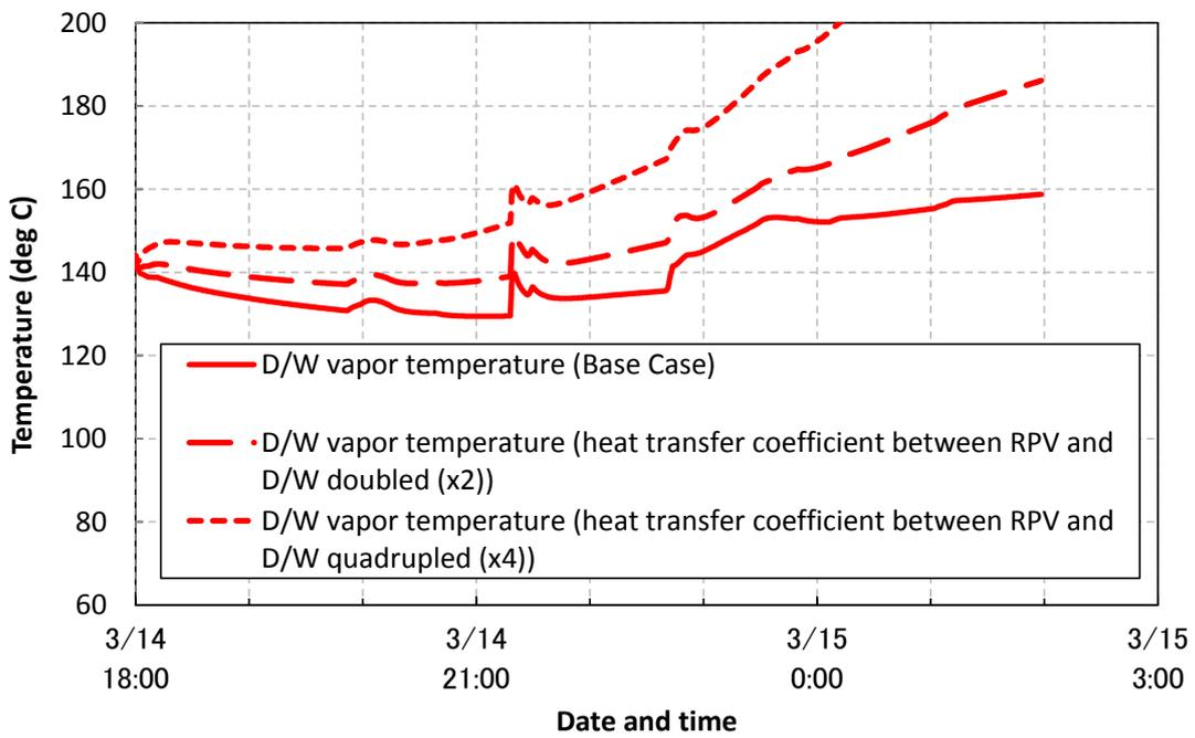
Figure 2.17 Results of Sensitivity Analysis Case ④ (D/W vapor temperatures)
