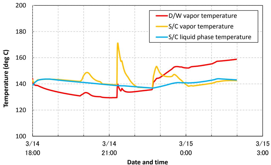
Figure 2-8 Base Case analysis results (PCV temperatures)
