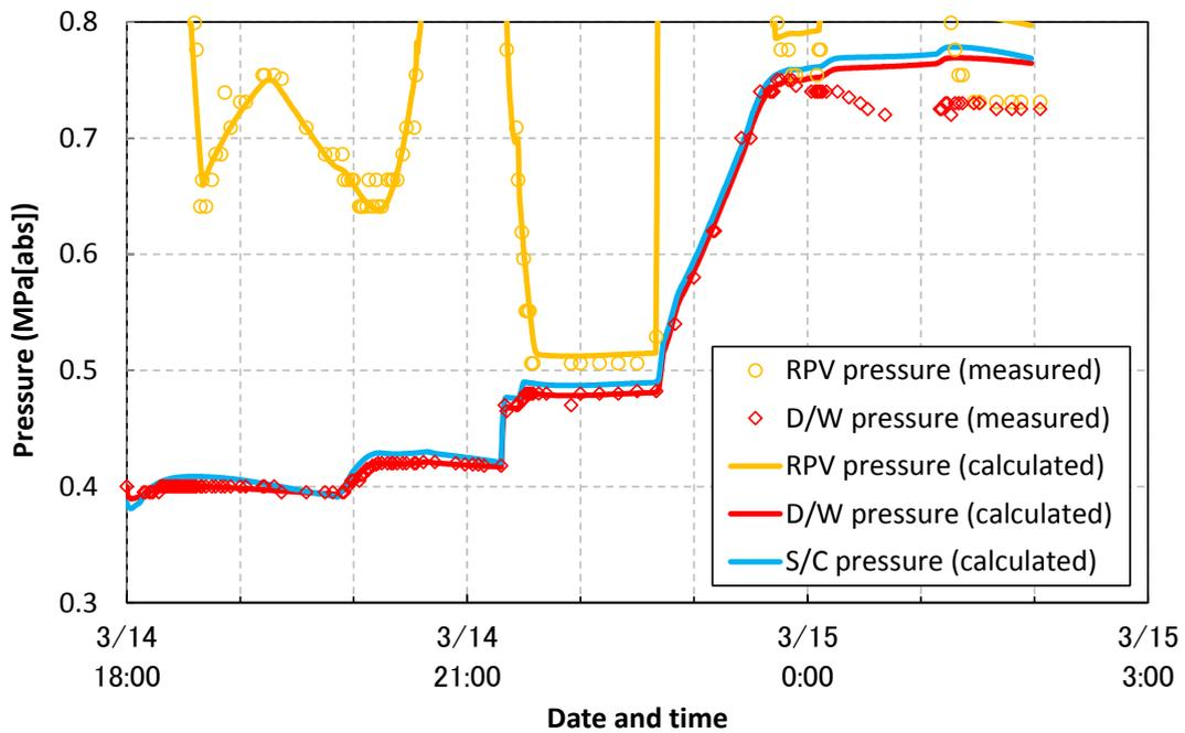
Figure 2.16 Results of Sensitivity Analysis Case ③ (pressures): 0.3 – 0.8 MPa
