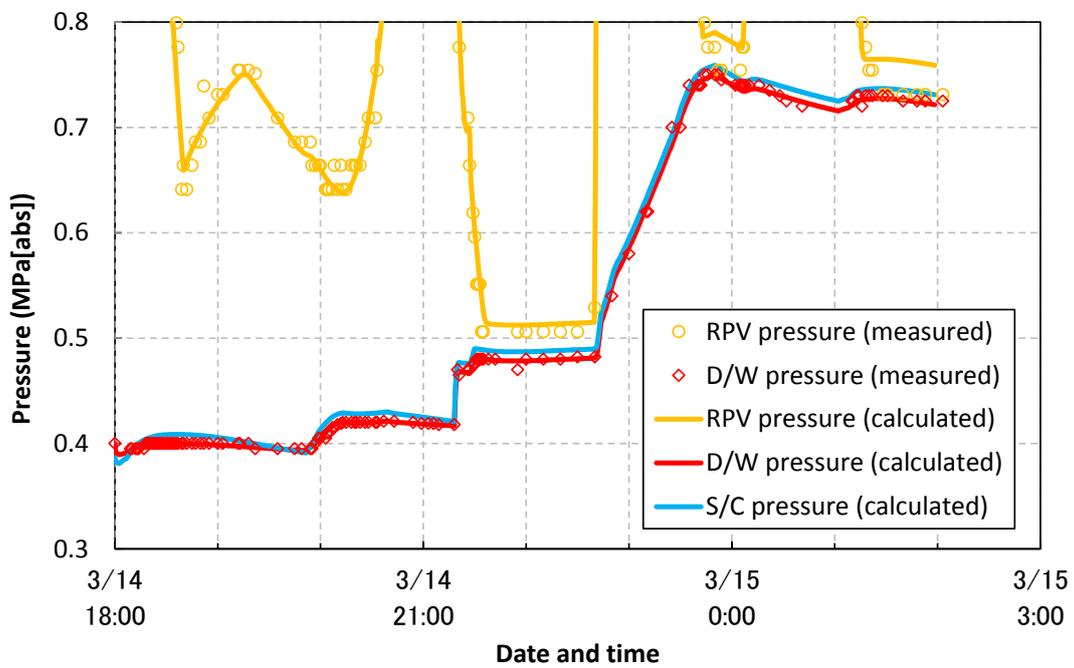
Figure 2-6 Base Case analysis results (Pressure): 0.3 – 0.8MPa
