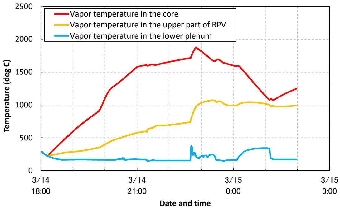
Figure 2-7 Base Case analysis results (RPV vapor temperatures)
