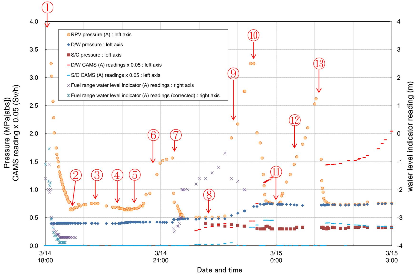
Figure 2.1 Measured data after Unit-2 forced depressurization
