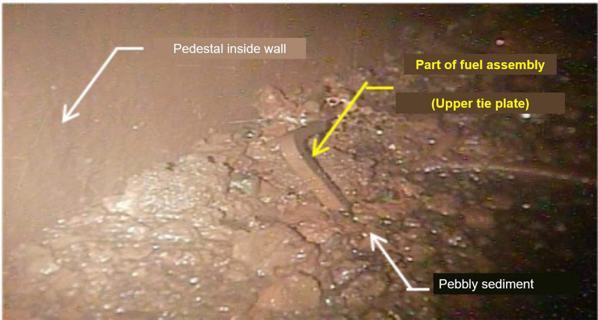
Figure 3-41 Sediments and dropped upper tie plate [3-19]
