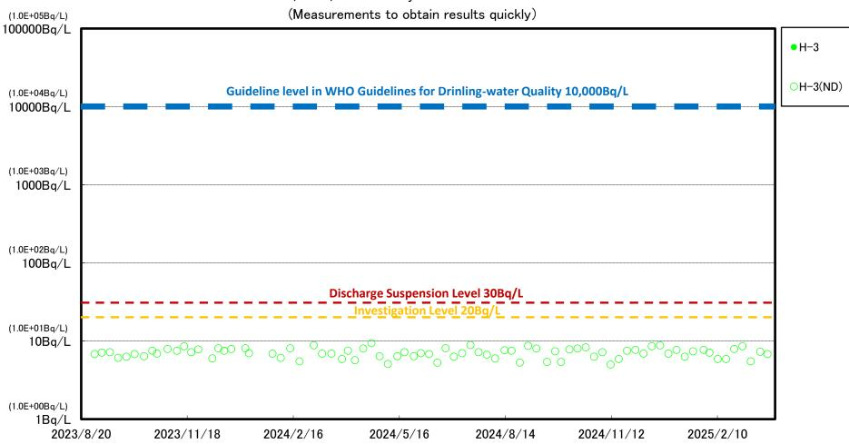
3km offshore of 1F site(T-D5) Surface layer Radioactive Concentration of Seawater
