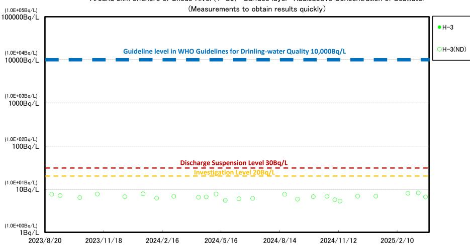
Around 3km offshore of Ukedo River (T-S3) Surface layer Radioactive Concentration of Seawater
