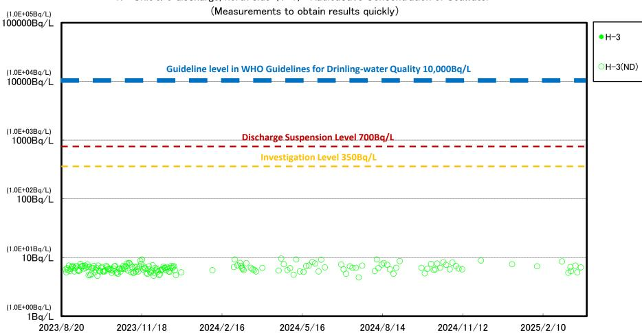
1F Unit 5/6 discharge, north side (T-1) Radioactive Concentration of Seawater
