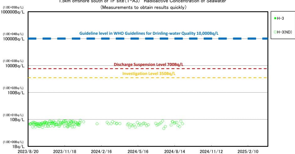
1.5km offshore south of 1F site(T-A3) Radioactive Concentration of Seawater
