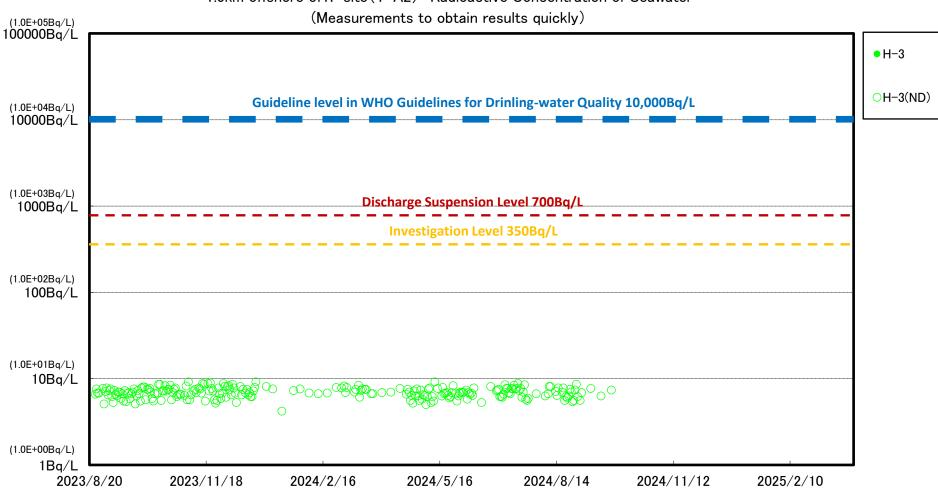
1.5km offshore of 1F site (T-A2) Radioactive Concentration of Seawater
