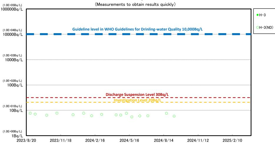
Around 3km offshore of 1F site(T-S4) Surface layer Radioactive Concentration of Seawater
