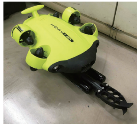
Small underwater drones utilized for hydroelectric power plant maintenance
