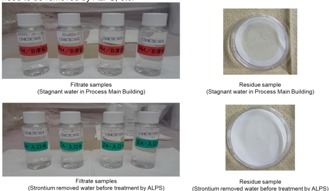
Figure I-17 Filtrate samples and residue samples from samples to be analyzed (stagnant water in Process Main Building and strontium removed water before ALPS treatment)
