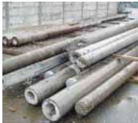
Dismantled concrete utility poles are sorted, nondefective poles to be reused.
