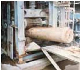
Defective poles are crushed, separated into steel and concrete.
