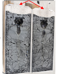
≈300 kg wasteform obtained after the first full-scale test with Dem&Melt (51wt% WL - STEP 3)
