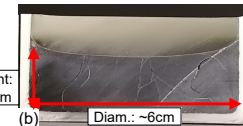
Example of lab-scale tests (~100g glass) (a): before the test, (b): after the test (51 wt% WL - STEP 3)
