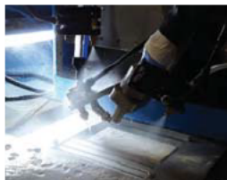
Fig. 3 Spray scrubbing test with laser cutting
