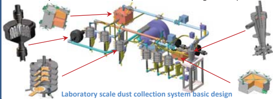
Laboratory scale dust collection system basic design
